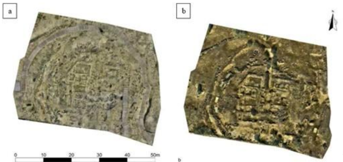
Figure 4: Orthophotos obtained from two photogrammetric survey techniques: a) network of oblique photos taken from a telescopic mast and utilizing an elevation model from TLS; b) vertical orthophotos using UAV. (Mozas-Calvache et al., 2012)
